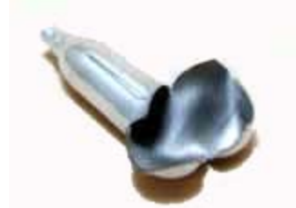
Figure 10: Powerlet ruptured by exposure to 180° F temperature in manufacturer’s test.
