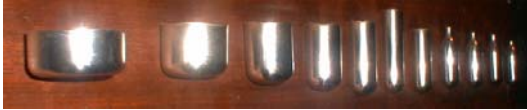
Figure 2: Evolution of the bottle shape from shallow cup to finished cartridge. Photo courtesy of Leland Limited
