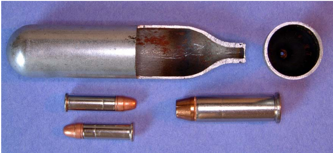
Figure 1: Sectioned 12 gram CO 2 cartridge shows thin (pierced) plug and far thicker walls. It is compared with two equivalent energy sources: two .22 Long-Rifles or one .38 Special.
